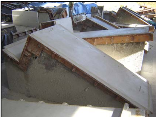
Figure 9 – GRC bed mould
