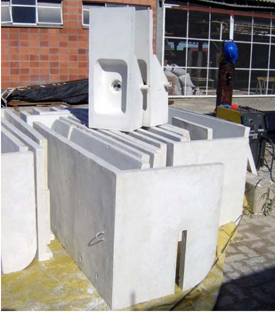
Figure 11 – GRC beds and washbasins made by Verdicon Construções Ltda, Canoas, Brazil
