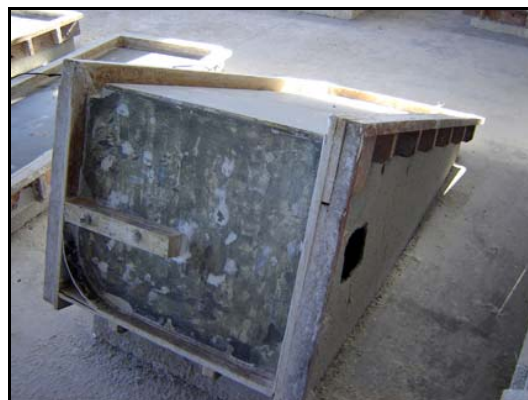
Figure 10 – GRC shelf mould
